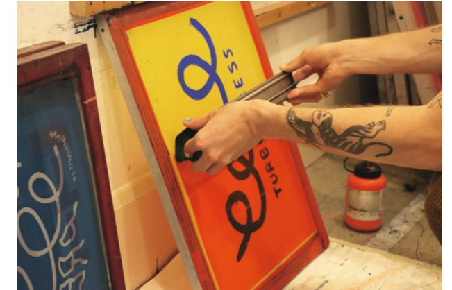
Employing Lascaux Screen filler, the negative of the motif is waterproofed.
