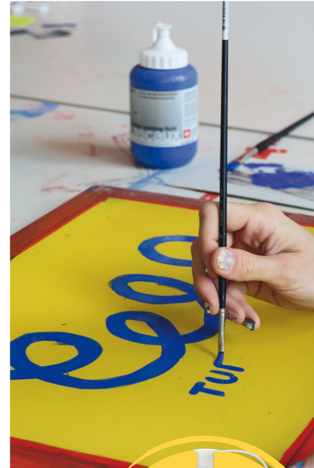
The positive of the motif is temporarily covered with Lascaux Screen painting fluid.
